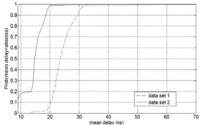
Figure 5. Experimental CDFs for mean delay.
