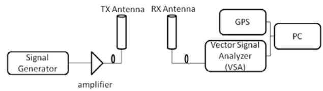
Figure 2. Block diagram of the measurement system.
