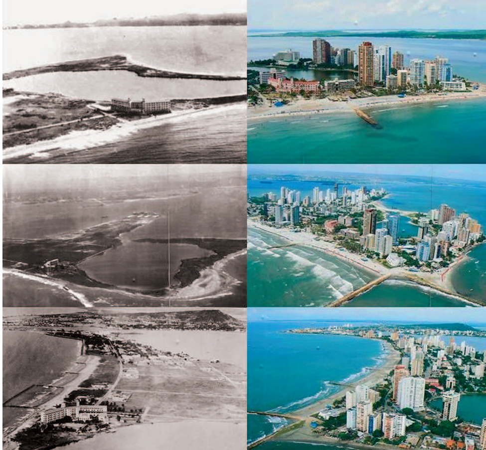
Fig. 2. Aerial view of coastal occupation and groin fields (“domino effect”) at Bocagrande, El Laguito and Castillogrande sectors (Cartagena City). The images on the left side correspond to 1950s, the ones on the right correspond to 2005 (courtesy of Historic Archive of Cartagena de Indias)
