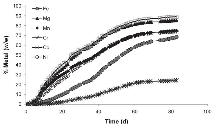
Fig. 6. Evolution of metals solubilised in the column leaching with CARON process residue (83% pulp density).
