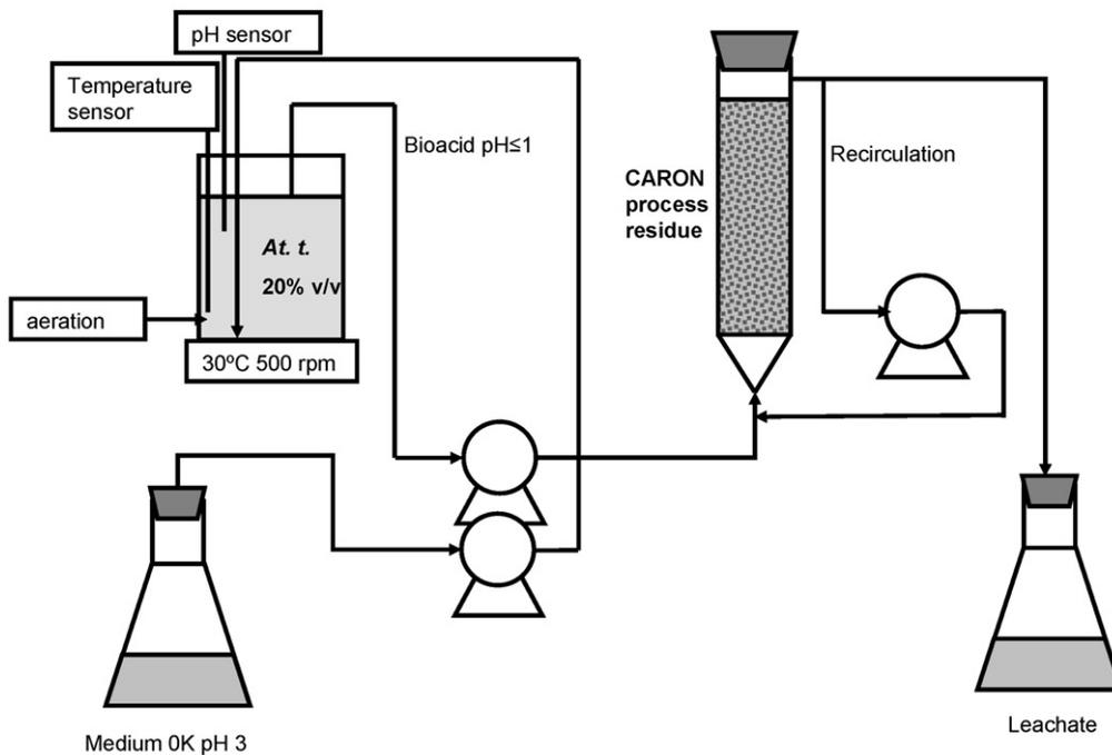
**Fig. 1.** Diagram of semicontinuous systems. (a) Bioreactor of *A. thiooxidans* connected with a stirred-tank reactor for leaching metals. (b) Bioreactor of *A. thiooxidans* connected with a column with recirculation for leaching metals.
