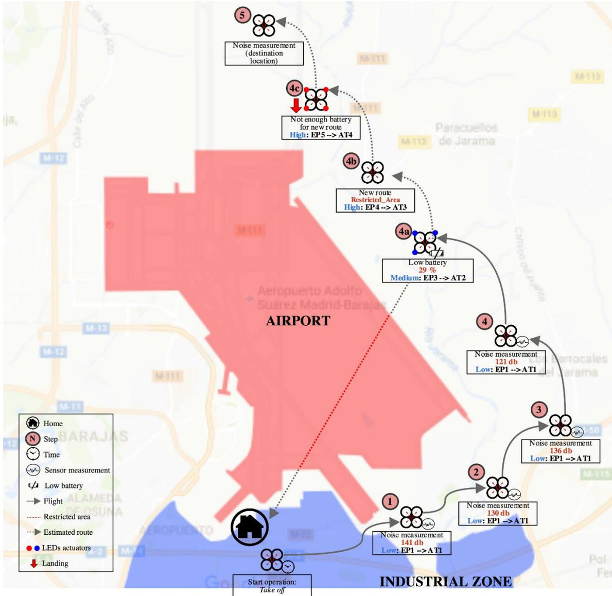
Figure 2. A practical example of applying the UAV real-time decision-making approach.
