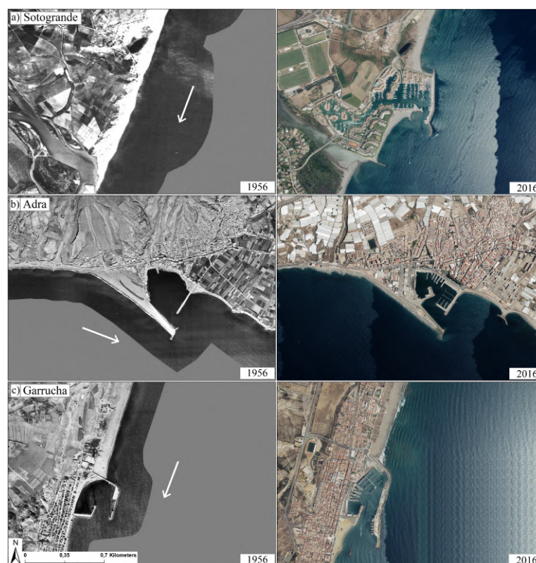
Figure 11. Examples of drift-and swash-aligned shoreline sectors. Stogrande Port (a) was constructed in 1987, Adra Port (b) in 1947 (the first emplacement) and the construction of Garrucha Port (c) started in 1931 and the last modification was carried out in 2009.
