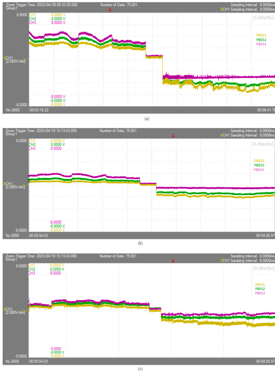
Fig. 17. Experimental results for BES power: (a) OPT-EMS, (b) SOC-EMS, and (c) MPC-EMS.
