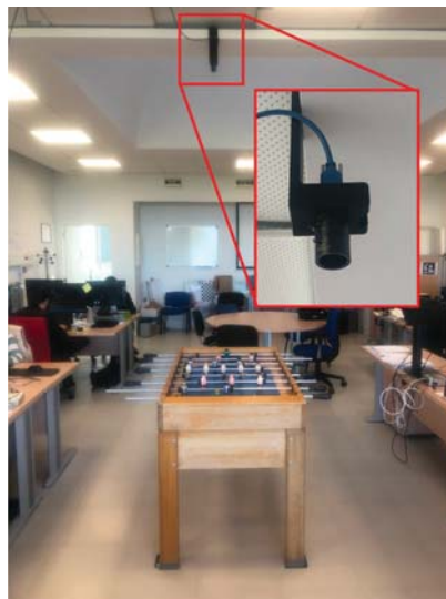
Fig. 2. The equipped laboratory to capture the trajectories of the ball with the event camera hanging from the ceiling.
