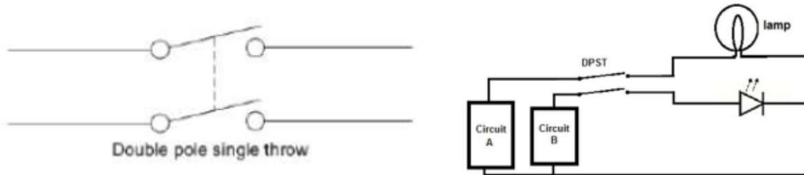
Double Pole Single Throw Switch (DPST) Circuit
