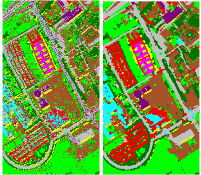
Fig. 8 SVM based pixel classification applied to the original hyperspectral image (left) and to the segmented image provided by the ECAS-II algorithm (right)
