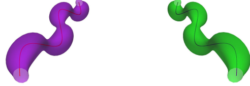
Figure 11: Basic flow plus perturbation for the leading mode at \tilde{k} = 0.8 comparison between the filament positions obtained from the vortex filament stability analysis at \tilde{d} = 0.1 (lines) and the vorticity isosurfaces obtained from the BiGlobal analysis for Re = 1000 and \tilde{a} = 0.1145 (surfaces). Perpendicular direction not scaled.
