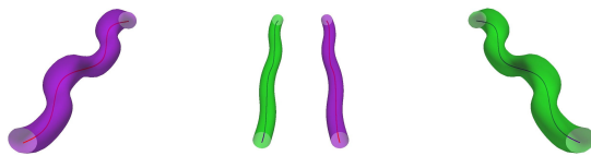
Figure 13: Basic flow plus \varepsilon = 0.02 perturbation for the second symmetric mode at \tilde{k} = 1.2 comparison between the filament positions obtained from the inviscid analysis at \tilde{d} = 0.02 (lines) and the vorticity isosurfaces obtained from the BiGlobal analysis for Re = 10000 and \tilde{a} = 0.0229 (surfaces). Perpendicular direction not scaled.
