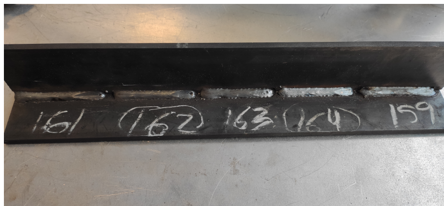
Figure 4. Steel plate where numbered seams were welded and then treated according to the experiment to be carried out.
