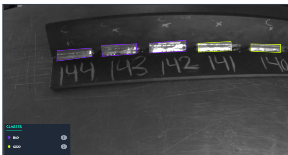
Figure 8. Mild steel plate with several welding beads, labeled with the online tool Roboflow, so that the system can detect a type of weld manufactured correctly compared to another weld manufactured with some defect.
