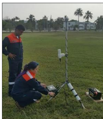
Figure 2. Installation of the Geometrics G-862 RBS Base Station.
