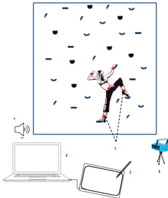
Figure 5. An illustration of different components of the system and their location consistent on (1) Inertial sensor, (2) Digital tablet/computer device equipped with a touch screen, (3) Personal computer/Data reception and acquisition system, (4) Sound emission system, (5) Laser projector.
