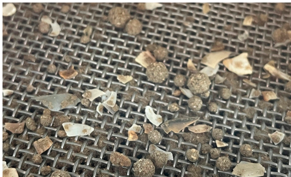
Figure 3. An example of a sieved sand sample that was not sufficiently dry. The sieving machine vibrations created compact sand spheres with the grains. Also, it can be seen how humidity in the sand causes obstructions in the mesh pores.
