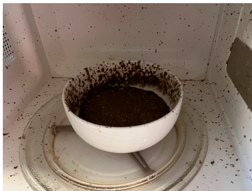
Figure 6. View of the inside of a microwave after a sand sample exploded during the drying process.
