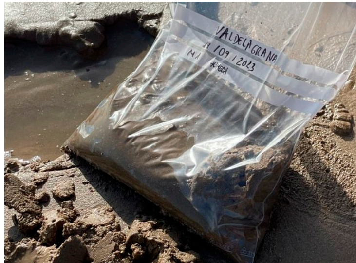
Figure 2. A sample bag (10 bags were collected from each beach) containing 800 g of sand with some excess water. Each sample bag was divided into 5 subsamples: 130 g for muffle, 130 g for each of the four microwave power levels (700 w, 595 w, 462 w, and 300 w), and 150 g extra for possible losses.
