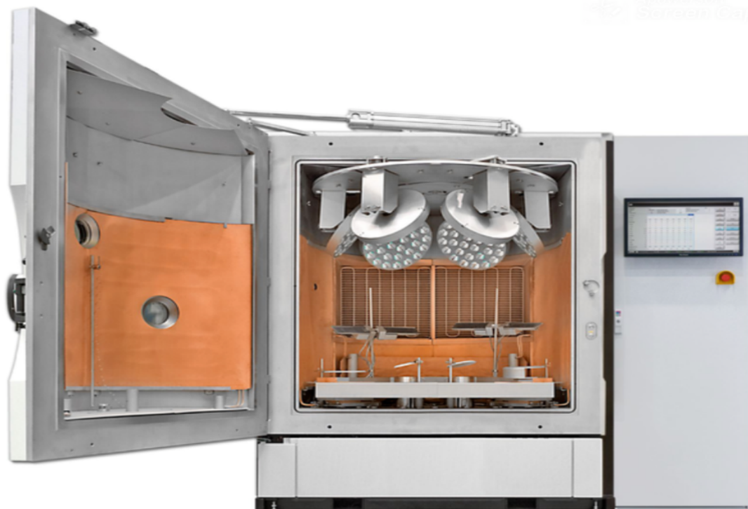
FIGURE 3.4: A Coater Machine by Bühler Leybold Optics for Air Coating Lenses. (©All rights reserved by Bühler Leybold Optics)
