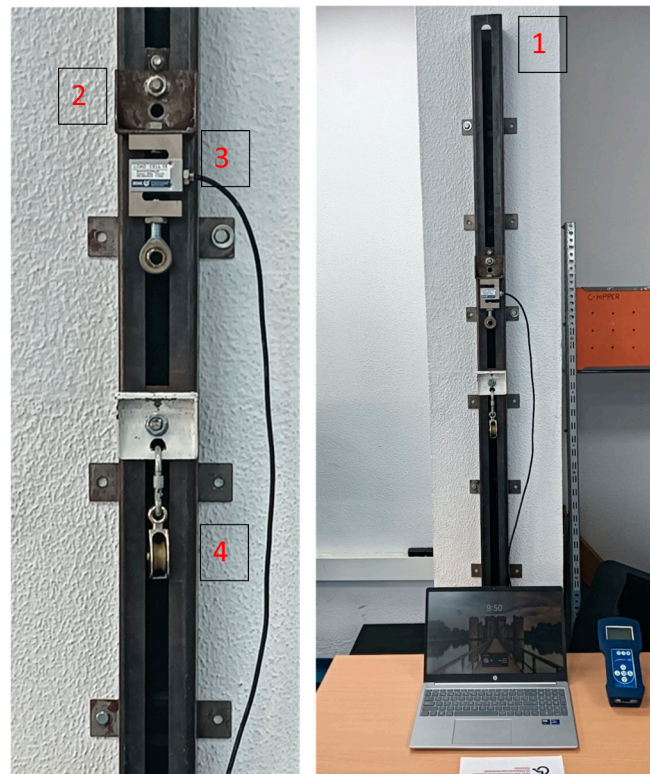
Figure 1. ISOMETRO system (University of Cádiz). Main components: (1) rail; (2) sled; (3) load cell; (4) optional transmission pulley for alternative force directions.
